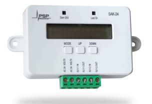
The SAK-24 provides a wireless solution to control loads of devices with dry contacts. The contacts are rated for up to 5 amps and 250 volts AC to control a broad range of applications. The SAK-24 is powered by 24 volts AC that can be derived from anywhere within the electrical systems. A connection or control wire back to the generator or transfer switch is not required.
