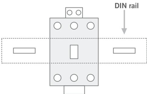
To attach contactor to din-rail insert flat bladed screw driver into slot and gently slide bar away from the contactor. Push down slightly on the contactor to lock in place on din rail.
