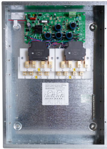
Includes Dual CTs for Precision Load Shedding Control
