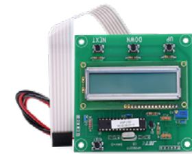
Easy-to-Use 3 Button Programming Module with LCD display
