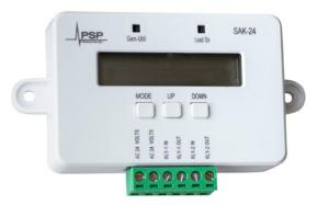
The SAK-24 provides a wireless solution to control loads of devices with form "A" dry contact. The contacts are rated for up to 5A and 250 VAC to control a broad range of applications. The SAK-24 is powered by 24 VAC that can be derived from anywhere within the electrical system. A connection or control wire back to the generator or transfer switch is not required.
