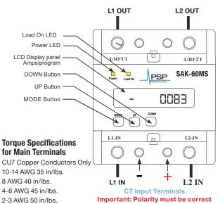
Push "Mode" button one time. Setup will begin by displaying setting "EF250". Each time mode button is pressed, the menu advances to the next setting. Adjustments to the settings are made using the UP & DOWN buttons. The program mode exits and saves settings after 30 seconds of inactivity. The reading on the display screen reflects the highest amperage recorded from either L1 or L2 from CTs. Technical Support Call **703-687-4057**.
