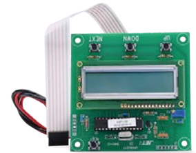
Easy-to-Use 3 Button Programming Module with LCD display
